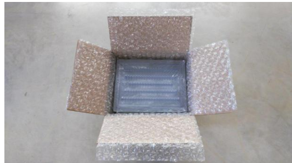
Picture - box with filling and packed product in group molding
